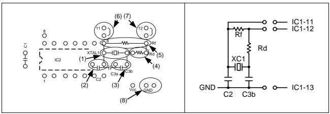
Figure 3 When using 2-pin type oscillator
